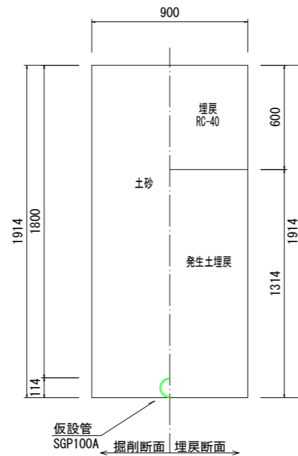
仮設土工2 撤去 (SGP100A DP=1.8m)
